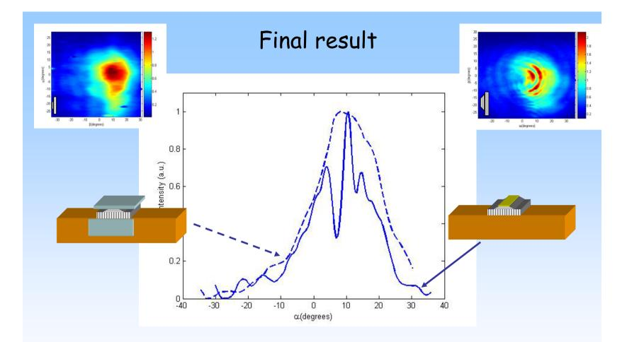
Terahertz absorber eliminate completely interference rings!!!
