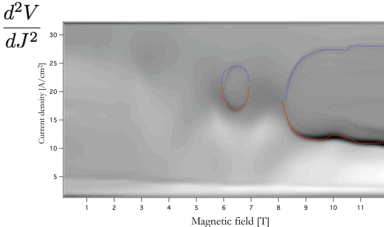
Very small laser ridge 550 μm long 100 μm wide: no change in threshold
