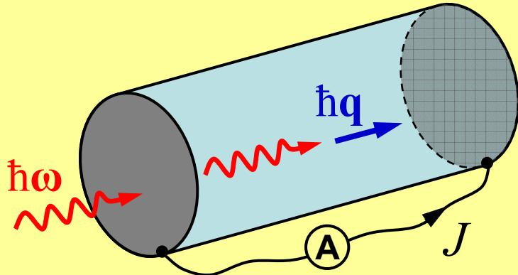
Photocurrent caused by transfer of photon linear momenta to free carriers
