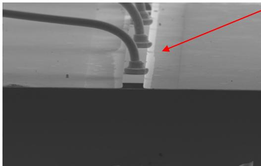
The relatively large width allows bonding directly on top of the ridge, whilst keeping a low capacitance thanks to the thick active region
