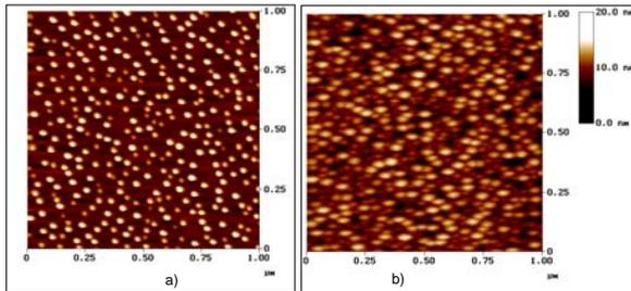
AFM images of :a) Standard In/GaAs dots, b) InAs on GaSb/GaAs dots
