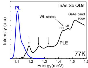
Photoluminescence and photoluminescence excitation for InAs in GaSb/GaAs dots
