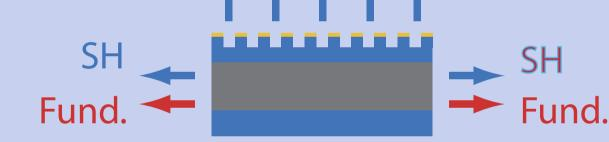
The grating was designed to be 1st order for the fundamental mode and hence it is 2nd for the SH mode. The device is only emitting SH via the surface.
