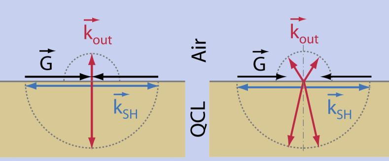
The phase mismatch and interference effetcs are mechanism for multi lobe emission as the SH wave vector does not perfectly match the 2<sup>nd</sup> order Bragg condition.
