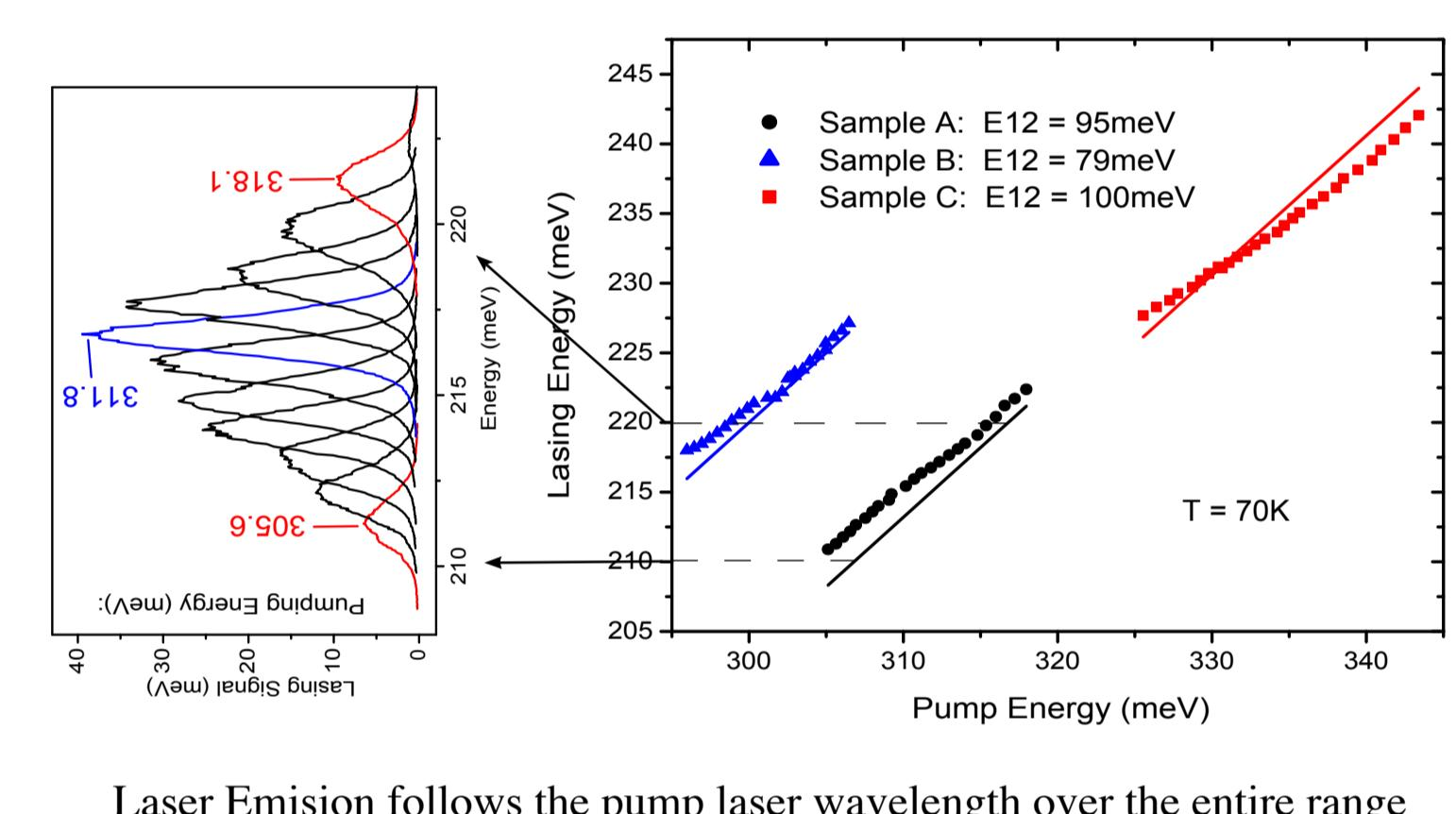
Laser Emision follows the pump laser wavelength over the entire range
