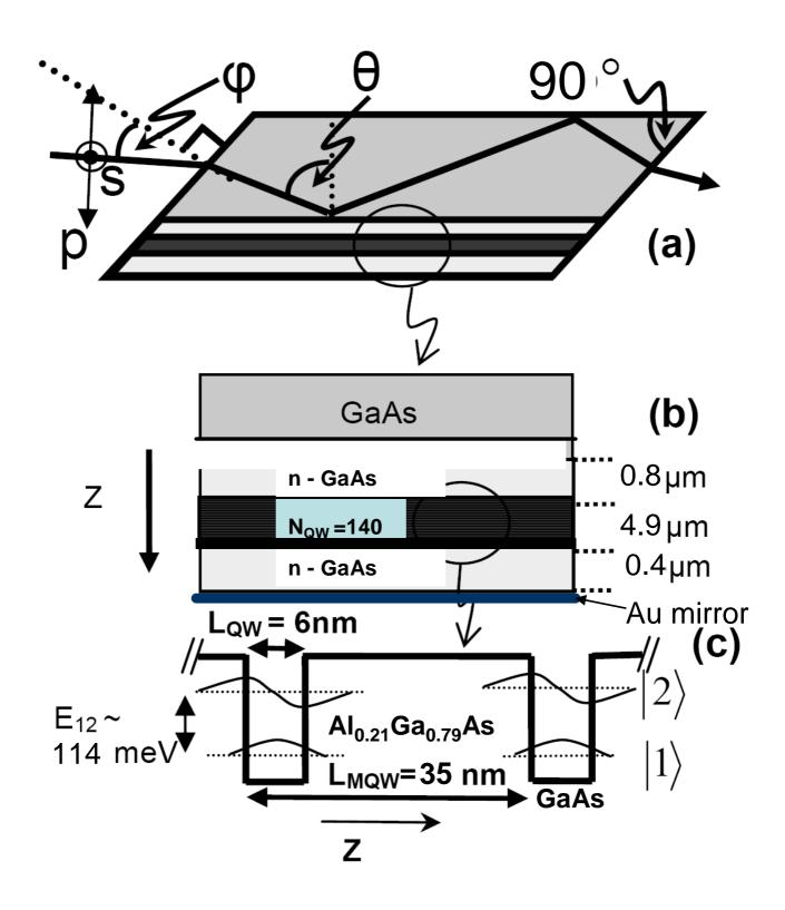
Figure 1: The prism coupling scheme (a) and the details of the metal clad microcavity structure studied in Ref. [1] (b,c).
