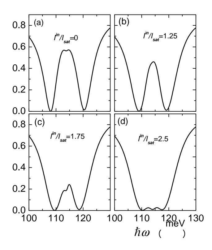
Figure 3: The spectral shape of R calculated for the structure presented in Fig.1 at different values of  $I^{\rm in}/I_{\rm sat}$ .  $N_s \times f_{12} = 2 \times 10^{10} \text{ cm}^{-2}$ ,  $\hbar \Gamma = 1.1 \text{ meV}$ ,  $\theta = \theta_{\rm res} = 73.2^{\circ}$ .
