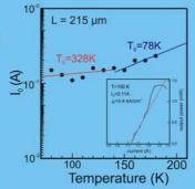
Comparison of threshold current of two identically processed devices with different cavity lenghts yield a mirror reflectivity of ~ 0.7
