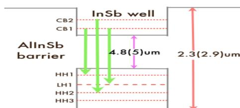
Energy separation at different levels and their corresponding wavelengths
